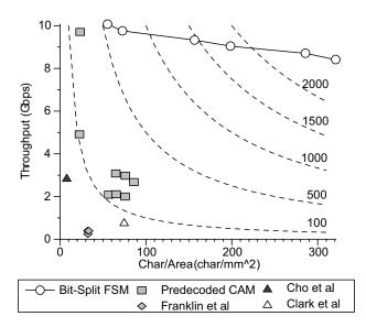
Figure 6: Efficiency (Throughput\*Char/Area) Comparison of String Matching Designs. Each dashed line is aggregation of all points that have the same performance per area value. The points on the upper right part denote more efficient designs. We can clearly see that even the least efficient configuration of our bit-split FSM design beats the best FPGA-based designs examined and most of the bit-split FSM design are far better than these FPGA-based designs.
